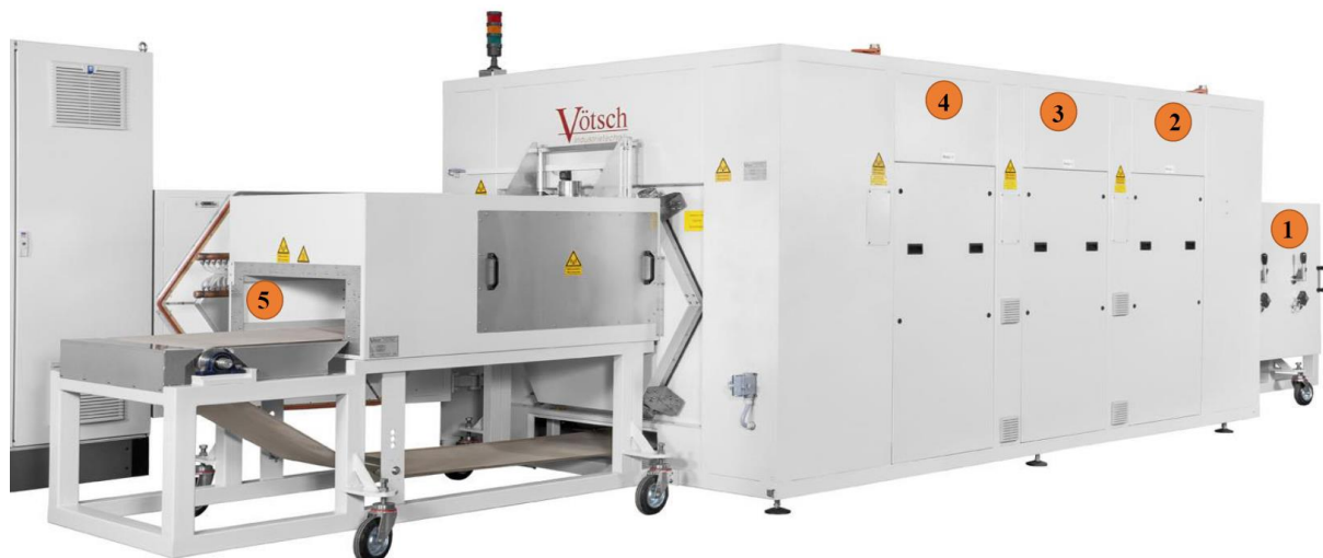
Fig. 15: A side view of the HEPHAISTOS microwave oven system. The main modules of the oven are represented by number tags 1, 2, 3, 4, 5. Tag 5 and Tag 1 represent the entrance of the wet foam and exit doors for the dry foam on the conveyor belt, respectively. Tags 2, 3, 4 indicate the three modular heating systems which inbuilt the hexagonal cavity with high power microwave heating sources and control system block. The MWT and ECT imaging modules are installed at the entrance (Tag 5) and exit (Tag 1) doors, respectively.
