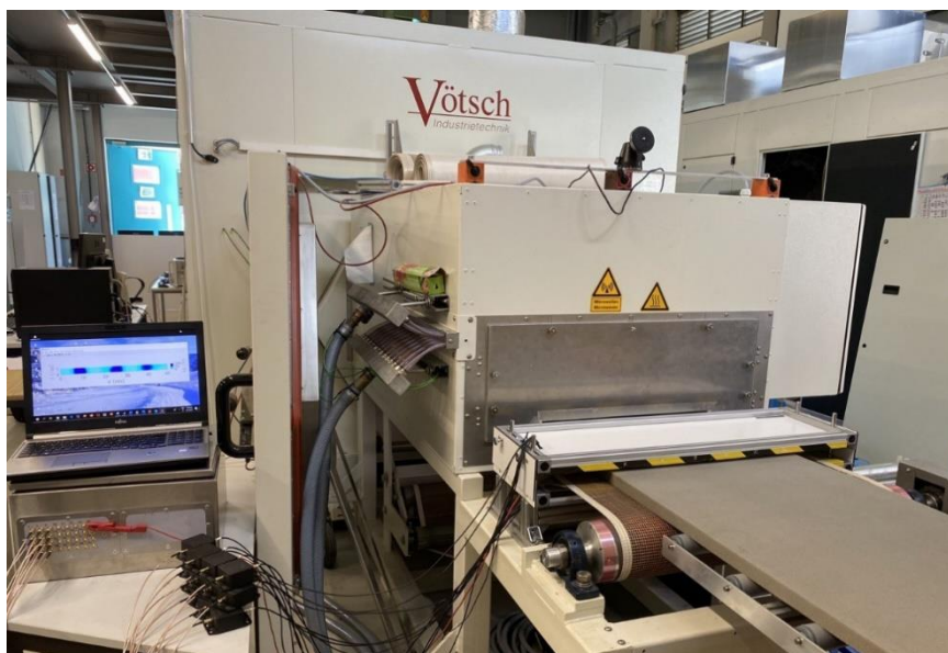
Fig. 18: The ECT sensor installed at the outlet of the HEPHAISTOS oven
