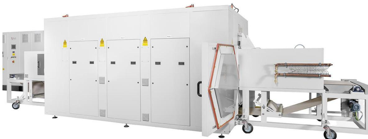
**Figure 5:** Photo of the industrial scale microwave system at KIT that will be used for the drying of porous foam in a continuous process
