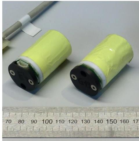
**Figure 16:** Gradiometric and absolute CIFT coil
