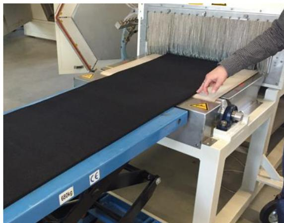
**Figure 6:** Photo of the industrial scale microwave system at KIT during operation with a continuous polymer foam from Pinta
