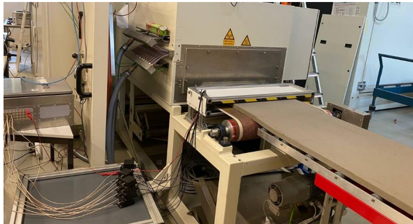
Fig. 38: The ECT sensor installed at the outlet of the HEPHAISTOS oven
