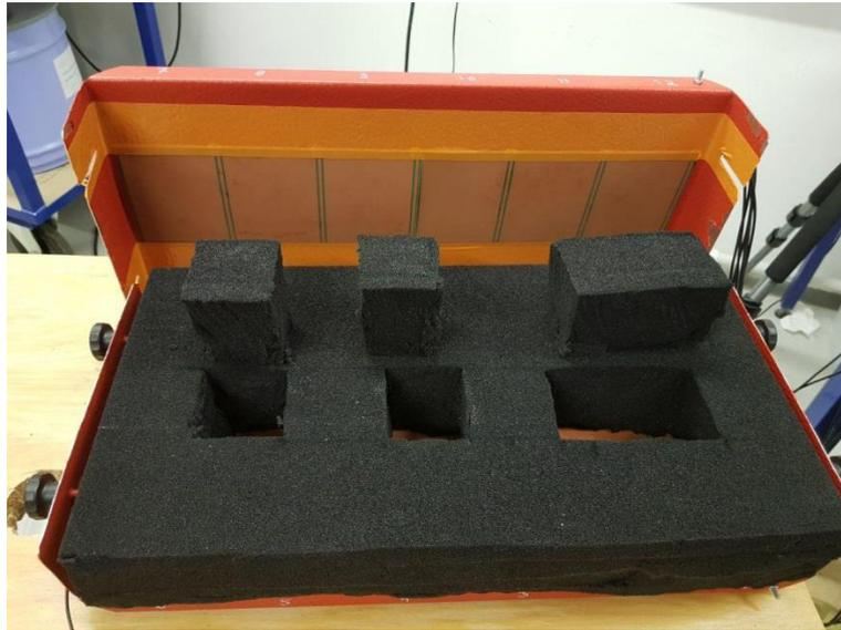
Figure 10: Experiment with ECT sensor by cutting three pieces of foam
