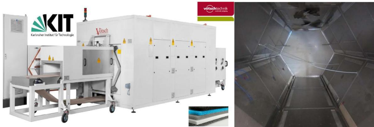
Figure 6: (left) Microwave HEPHAISTOS oven, (right) inside the oven with the hexagonal cross section
