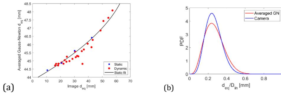
**Figure 3.** (a) Average equivalent diameters obtained using the Gauss-NewtonGN reconstruction scheme plotted against the camera values for the static and dynamic experimental points. (b) PDF of the equivalent core diameter -to- pipe inner diameter ratio for 1 experimental point.
